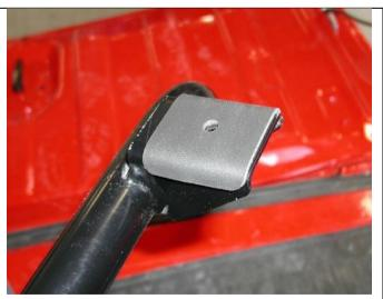
1. Fit seals, (4 OFF) to the brackets welded to the internal tube frames as shown.
