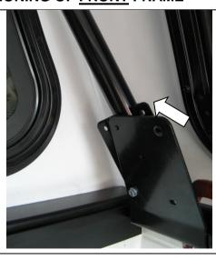
1. Fit on "U" shaped clamp bracket (6582434) in one corner, as shown, using one:
