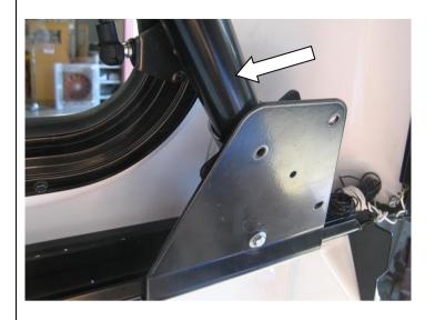
1. Fit on "U" shaped clamp bracket (6582434) in one corner, as shown, using one:
