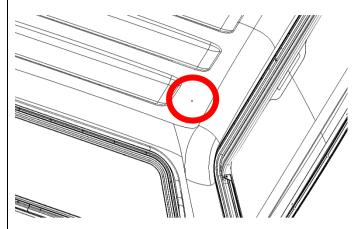
Locate the 4 moulded in roof dimples at the front and rear inside the canopy shell and using a 25mm hole saw cut holes through the shell from the inside using the dimples as drill point centre.
